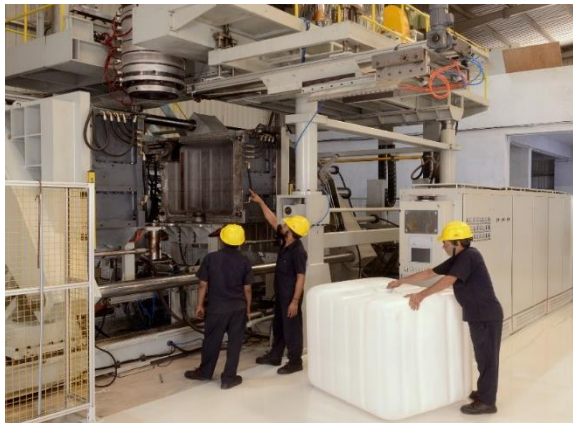
Manufacturing of rigid Intermediate Bulk Containers
